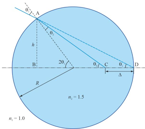
Consider the general geometry shown in the above figure. A light ray incident upon a sphere, of refractive index  $n_2$  that is different from that of the ambient  $n_1$  and a radius  $R$ , will intersect with the reference axis passing the center of the sphere at a shifted location by a distance  $\Delta$  from its original intersection point of distance  $R$  from the center. From simple geometry, we have
